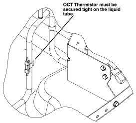
Fig. 9 - Outdoor Coil Thermistor (OCT) Attachment
